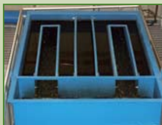
Close-up of plate settler
